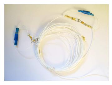
now have a 30m dipole. If I disconnect the closest connectors to the bnc connector, it's a 20m dipole.
